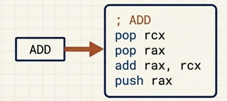
Each simple stack operation is mechanically translated into a sequence of concrete machine instructions.
